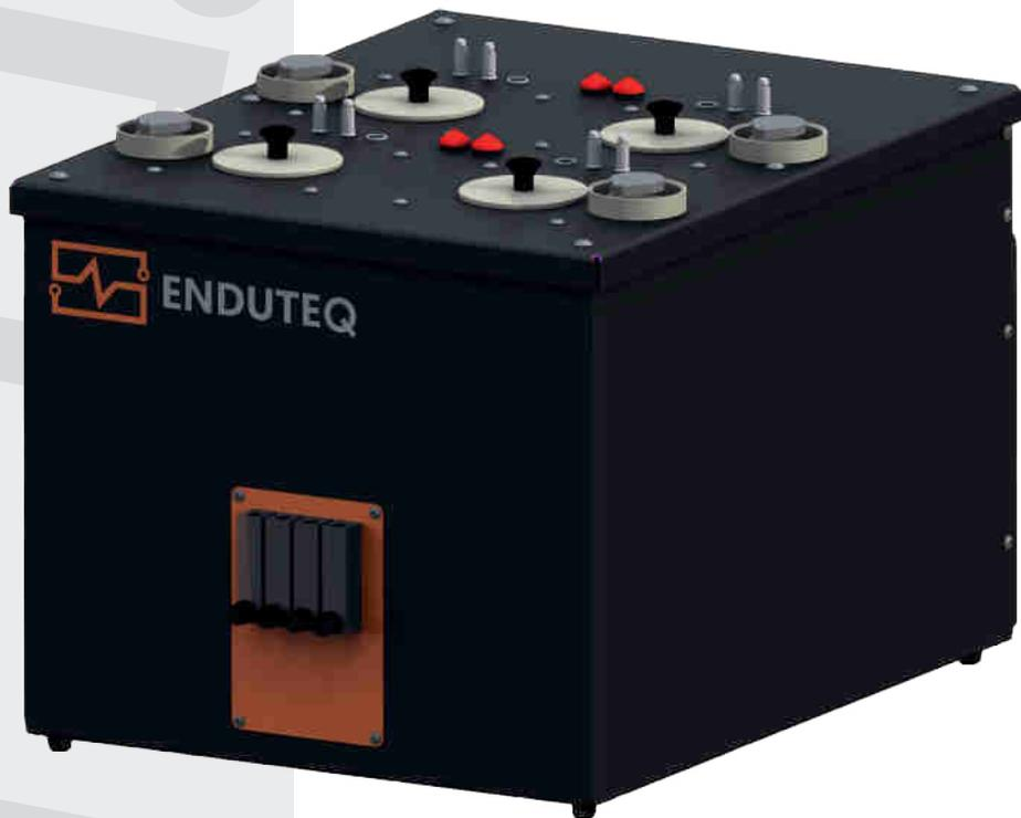
**A Stress relaxation test system conducts tests on rubber materials according to ISO 3384-1 and 2 norm.**
